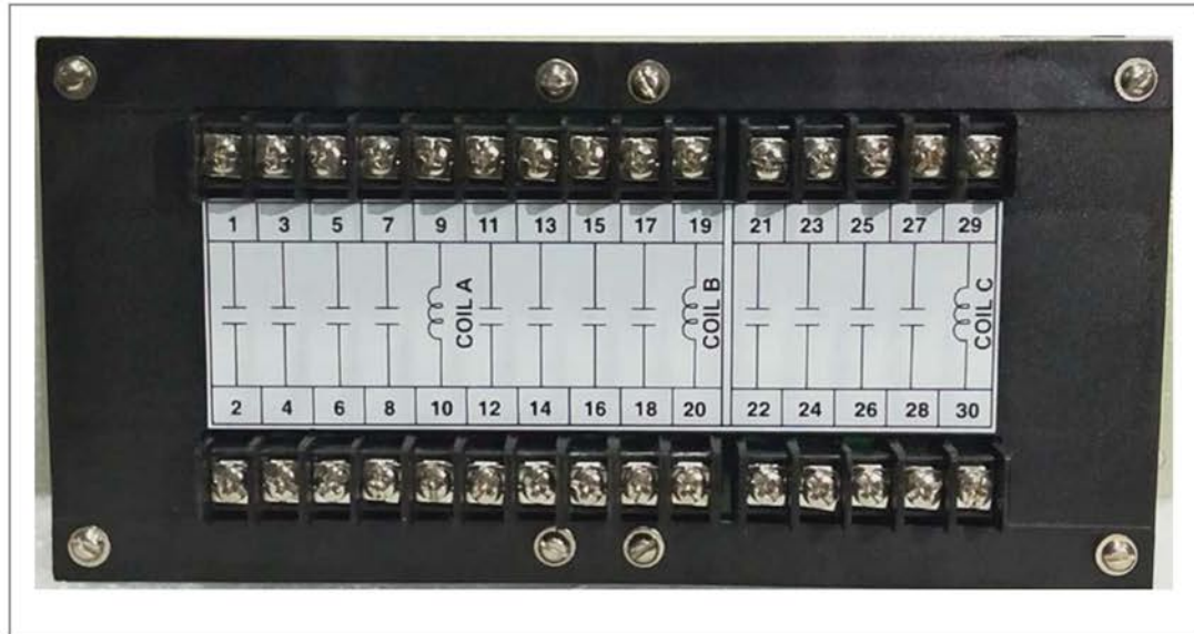
Figure 3: Relay back terminal view
